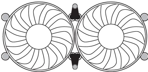
Dual fan mount using nylon tie rods
