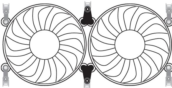
Dual fan mount using Splined ratchet brackets
